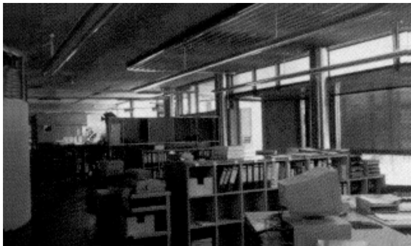
The Geysel office building in Cologne, Germany, is one of the case study buildings. This building has a special daylight guiding system directing sunlight to the ceiling to illuminate rooms using natural daylight without glare and reducing the use of artificial lighting
