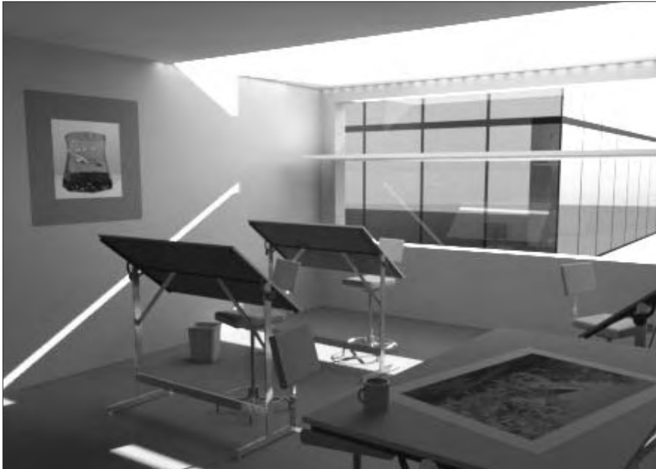
Figure 2. Example of a Radiance rendering of an office with a light shelf.
