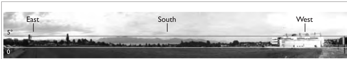
Figure 4. Panoramic view of the horizon as seen from the windows of the test rooms, when facing due South. For comparisons of the daylight conditions in the test room and the reference room, the exterior conditions must be almost identical, preferably with no obstructions. In this case, the angular altitude of external obstructions is lower than 5°.
