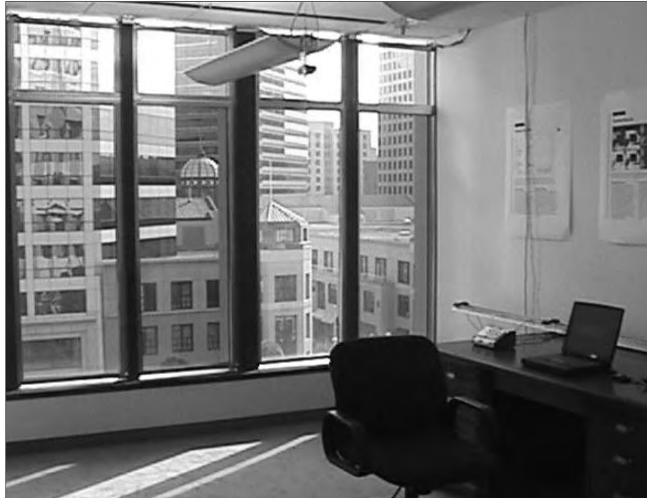
Figure 5. Interior view of the Oakland Federal Building testbed with electrochromic glazings installed.
