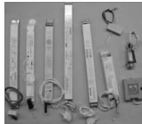
Samples of Subtask B daylighting system components: ballasts, sensors and controllers used in Subtask B.
